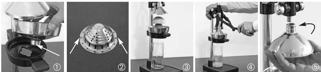
Place the funnel into the fitting of the pomegranate-juicer. Pay attention to the according gaps (picture 1). To fix it, turn the funnel slightly to the left or right. Fix the cone in the funnel and again pay attention to the gaps (picture 2).
